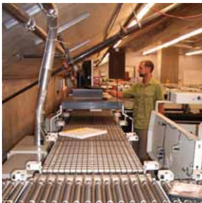
Seattle Main: RFID tags are read by scanners and sorted for distribution.
