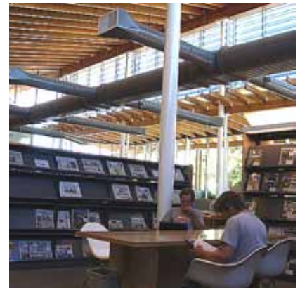
Ballard Library: inside clerestory windows help push light deep inside the space and balance daylight at perimeter.
