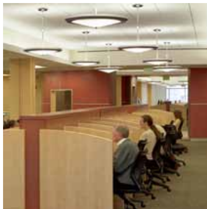
Doyle Library: a combination of indirect cove lighting and direct-indirect pendants provide glare free lighting for computer stations.
